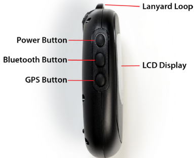
Figure 3 - Side View of the GNSS Surveyor
