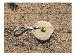
Since ESRI Collector is connected to the Bad Elf Bluetooth GPS through the iPhone, data can easily be added to the Bad Elf collection layer. After placing the GPS on the monument, allow the satellite reading to stabilize for a minute to acquire a better positional accuracy. Satellite coverage can be viewed in the Bad Elf app.
